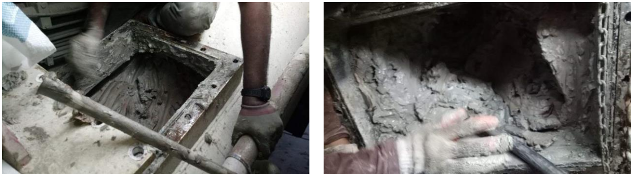
Fig. 13 Clogging of screw conveyor due to stickiness of clay
